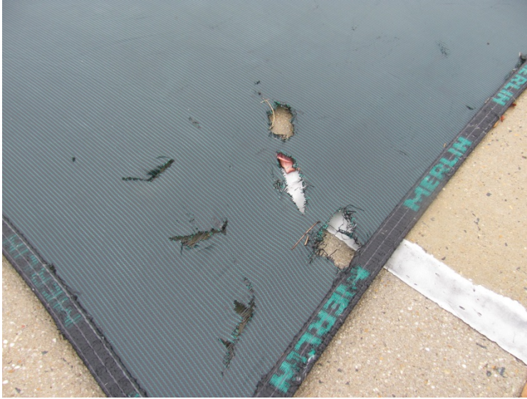
Vinyl cover damage
